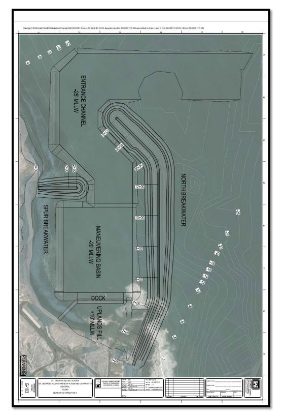
Figure 2. Recommended Plan – Conceptual Plan View Drawing
